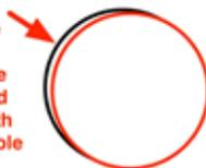
Align the engraved ring (shown in red) on the template with as much shot hole curvature as possible. If the shot hole curvature extends very slightly outside of the engraved ring, that is evidence of a double.
